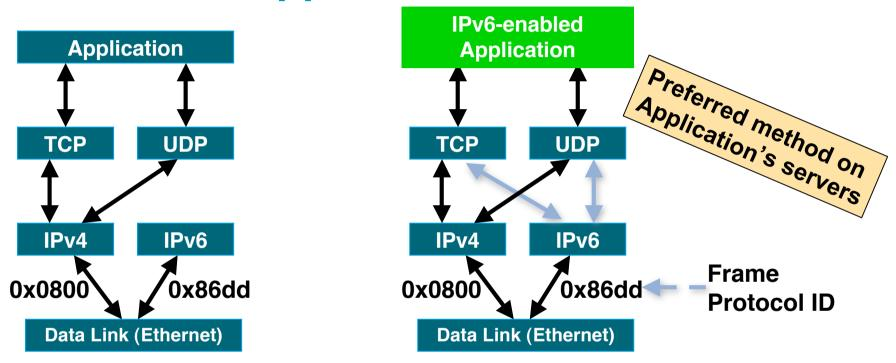
Dual stack node means:
