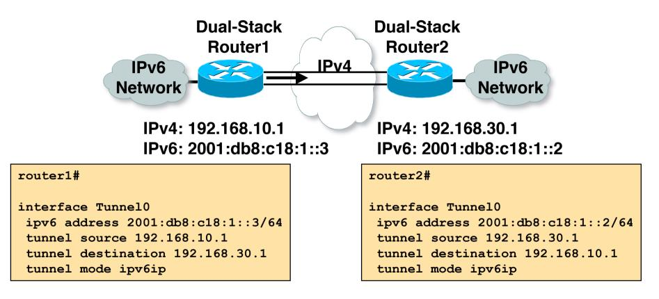
Manually Configured tunnels require: Dual stack end points Both IPv4 and IPv6 addresses configured at each end
