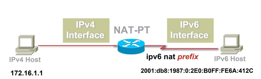
prefix is a 96-bit field that allows routing back to the NAT-PT device
